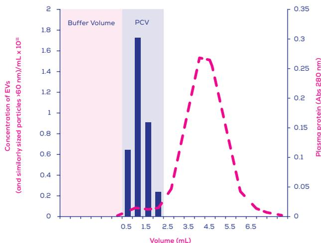
**Figure 5:** Typical elution profile for a qEVOriiginal column with 0.5 mL of plasma loaded; proteins elute later than extracellular vesicles (EVs) and similarly sized particles >60 nm. Particle concentration was measured using TRPS and protein levels by absorbance at 280 nm.
