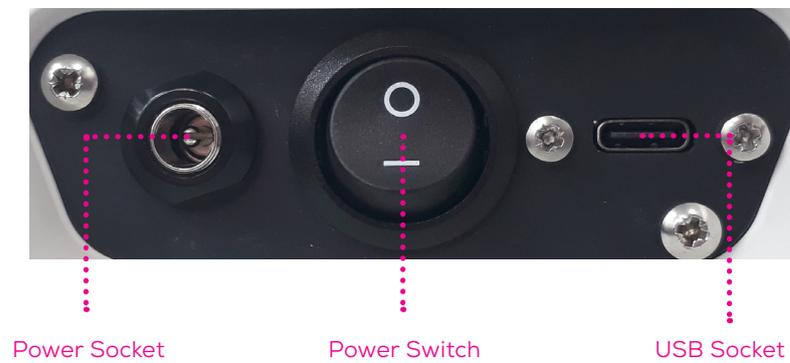
**Figure 8:** Switches and sockets on the Exoid.
