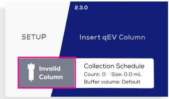
Figure 13: The home screen displaying the error message when a column has been used 10 times.
