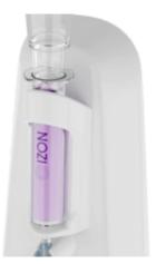
Figure 10: A qEV original/70nm Legacy column loaded correctly onto the AFC(V1). Ensure that the IZON logo is facing away from the AFC(V1) tower.
