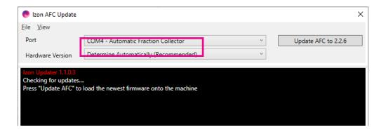
Figure 20: The Izon AFC(V1) Update software with the AFC(V1) correctly selected in the "Port" dropdown box.
