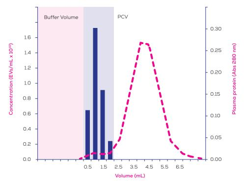
Figure 1: Typical elution profile for the qEVoriginal. Larger extracellular vesicles (EVs) and exosomes elute first, while smaller vesicles and protein complexes elute later;  $500~\mu L$  of bovine plasma on a qEVoriginal; concentration of EVs measured with a qNano and TRPS; concentration of proteins measured with spectrophotometry.
