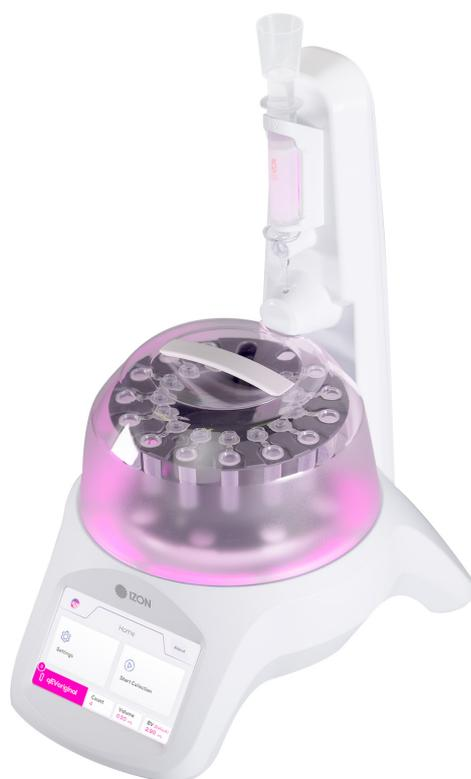
The AFC measures the volume of each fraction by weight as it fills with liquid eluting from the column. When the designated threshold weight is reached, the fluid flow is automatically stopped to prevent dripping of fluid during repositioning of the carousel.
