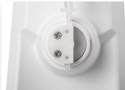
Figure 24: Pinch valve cover removed; pull tube laterally.
