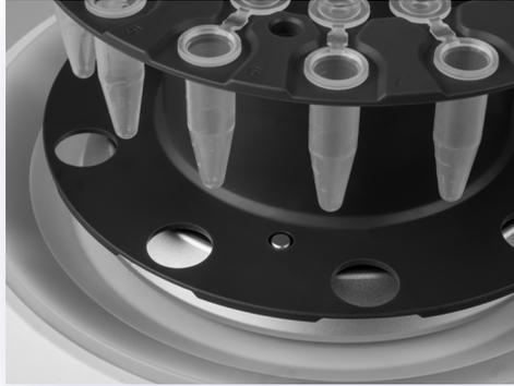
Figure 19: The alignment pin correctly engaged in the carousel.
