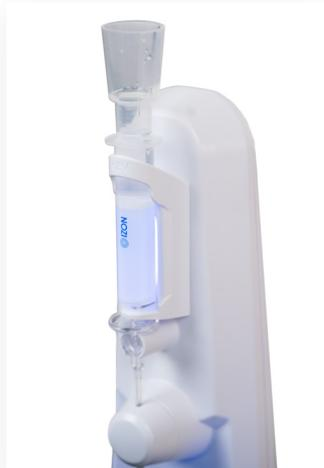
Figure 9: A qEVoriginal/35 nm Gen 2 column loaded correctly onto the AFC.
