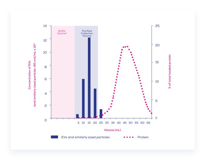
Figure 2. Typical elution profile for qEV10/35 nm Gen 2 columns with 10 mL of human plasma loaded; proteins elute at a later volume than extracellular vesicles and similarly sized particles >60 nm. EV concentration was measured using an Exoid and protein levels by bicinchoninic acid (BCA) assay. \*Recommended buffer volume values vary for qEV10/35 nm and qEV10/70 nm columns: refer to your qEV User Manual for guidance.
