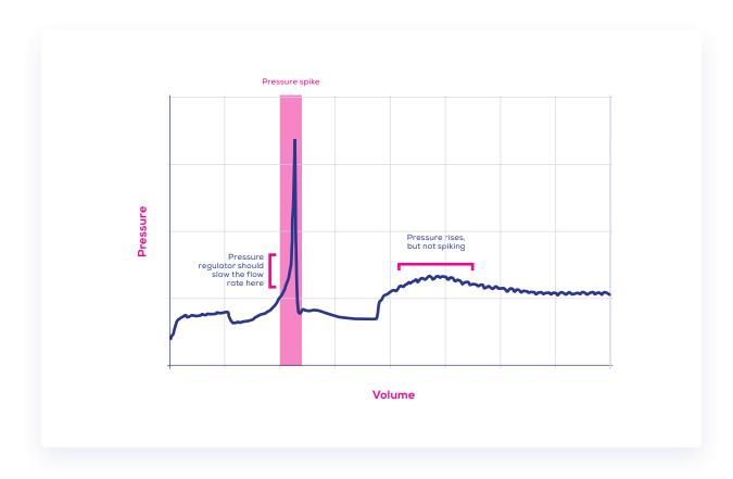
Figure 3. Column pressure without the use of pressure regulation.
