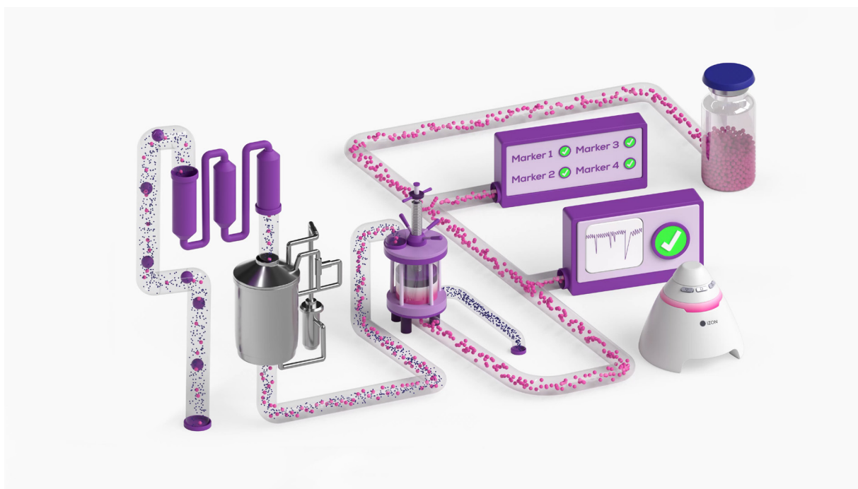
Figure 4. An exemplar, conceptual qEV PurePath workflow for therapeutics. Step 1 is clarification, which for automated systems is most likely to be in the form of serial filtration steps to eliminate larger contaminating particles. Next we have concentration, for which we recommend our tried and tested tangential flow filtration solution. After concentration, it is time for isolation in the form of a fully customised size exclusion chromatography column based upon qEV technology. Next come quality control steps, where particle size, concentration and zeta potential can be measured using Tunable Resistive Pulse Sensing, followed by assessments of potency and reproducibility (using assays built in partnership). Finally, you store the final, well-characterised and pure product. Pink = EVs; blue = protein; purple = large contaminants.
