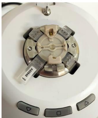
Figure 5: Nanopore securely attached to the stretcher jaws.
