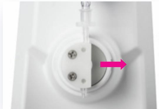
Figure 22: Pinch valve cover removed: Pull tube laterally.
