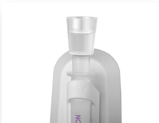
Figure 18: A column reservoir on a qEVoriginal column.
