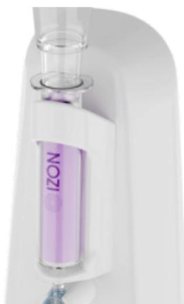
**Figure 10:** A qEV original/70nm Legacy column loaded correctly onto the AFC(V1). Ensure that the IZON logo is facing away from the AFC(V1) tower.
